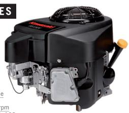
726cc V-Twin Four Stroke Engine Max Torque 53.9Nm @ 2200rpm 1½" Shaft, length 108mm Cast Iron Cylinder Liners Electric Start Weight 40.0kg (dry)
