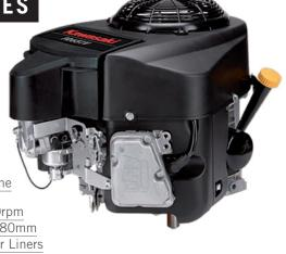
21.5hp 726cc V-Twin Four Stroke Engine Max Torque 53.3Nm @ 2200rpm 1" Shaft, length 80mm Cast Iron Cylinder Liners Electric Start Weight 40.0kg (dry)
